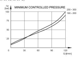
P-T pressure drops with screw set at minimum pressure control
