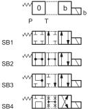
Type **TB**: 1 solenoid side B 2 external positions with return spring
