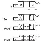
Type SB\*: 1 solenoid side B 2 positions (central + external) with spring centering
