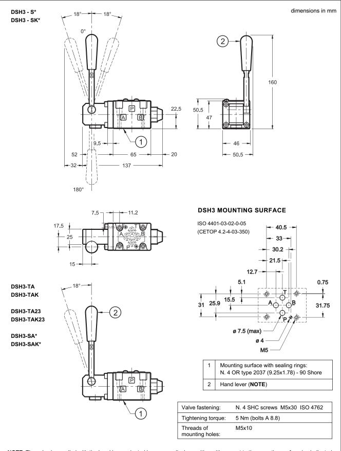
**NOTE**: The valve is supplied with the hand lever oriented in a perpendicular position with respect to the mounting surface (as indicated in the above drawing). For installation needs the hand lever can be oriented by the user directly at 180° to the standard position, simply by unscrewing the lever and re-screwing it in the desired position.
