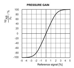
The diagram on the left shows the valve pressure gain, expressed as % of the ratio between the port pressure variation in A or B ( $\Delta p$  AB) and the P system pressure, according to the reference signal. Practically, the pressure gain states the valve reaction towards external disturbances aimed at changing the actuator position.
