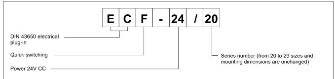
The ECF connector is a digital amplifier controlling open loop on-off valves.
