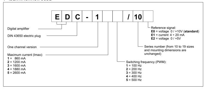
The EDC-1 connector is a digital amplifier controlling open loop proportional valves. The unit supplies a variable current proportionally to the reference signal and independently of temperature variations or load impedance, with a resolution of 1% on 2600 mA (the full scale value).
