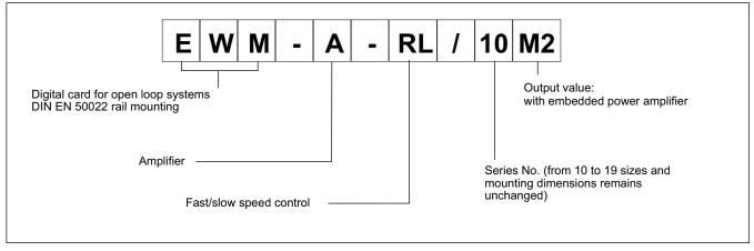
The power amplifier is controlled by an enable input and three switch signals. Therefore 8 demand values can be activated binary.
