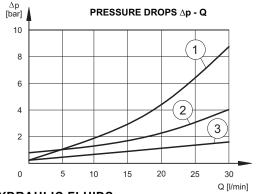
Typical  $\Delta p$  - Q curves obltained with QTM2-D valve, with throttling axis at full retraction.
