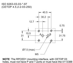
holes, must not have P and T ports or must have the 0113388 subplate (see paragraph 9)
