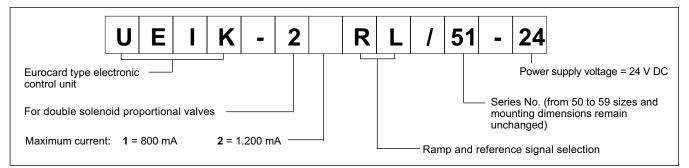
The UEIK-2\*RL card is an electronic control unit in Eurocard format for open loop control of double solenoid proportional valves, with selection in sequence of four different reference and ramp time regulation signals.
