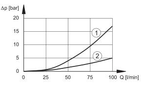
1) pressure drops  $P_1 \rightarrow P$  and  $T \rightarrow T_1$  (controlled lines)
