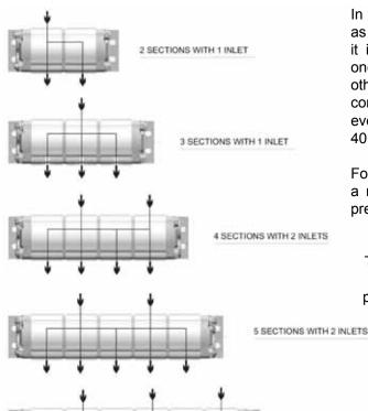
In flow dividers with many inlets, as they are all communicating it is even possible to use only one of them, by plugging the other ones. We suggest to make configurations with one inlet every 80 l/min (for 2DRE) and 40 l/min (for 1.5DRE) of flow elaborated.
