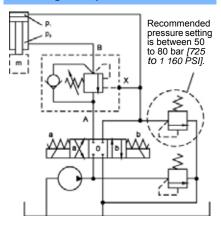
Because of the multiplication of pressure in hydraulic cylinder by the difference of surface areas:
