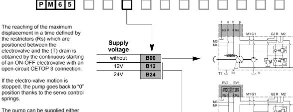
The pump can be supplied either without electrovalve (B00) or with electrovalve (B12, B24).
