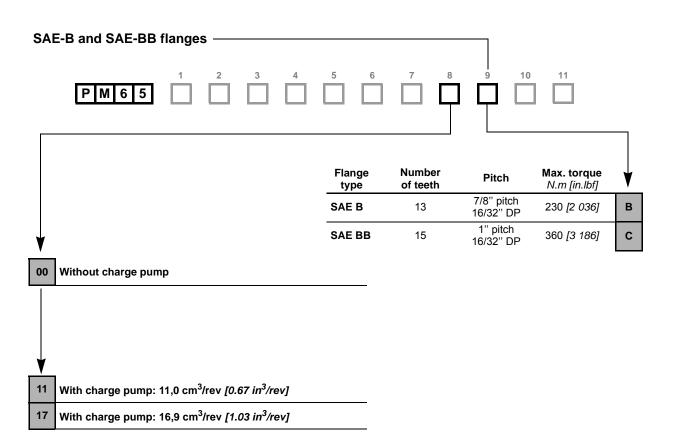
Splined ANSI B92.1a-1970 5/8" Pitch 16/32" DP Pressure angle 30° Tolerance class: 5
