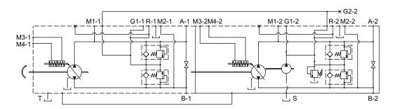
Ports T and G of the first pump must be connected with ports T and G of the
