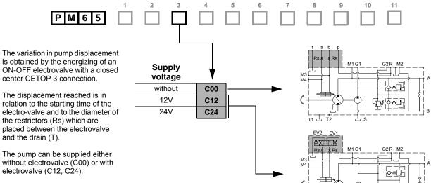
The pump can be supplied either without electrovalve (C00) or with electrovalve (C12, C24).
