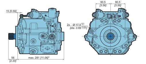
All length dimensions of pump body with different auxiliary mounting pads are shorter compare to standard 4-bolt flange of 14 mm [0.55 inch].
