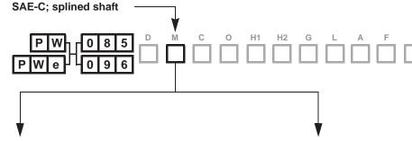
2 21 teeth; Shaft torque: 820 Nm [7 258 in.lbf] (without radial force)
