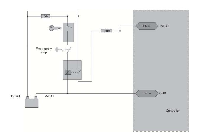
The correct wiring of the power supply pin (+VBAT) and pin connected to ground, is shown in previous figure. Power supply must be connected through an automotive fuse SAE J1284 20A.
