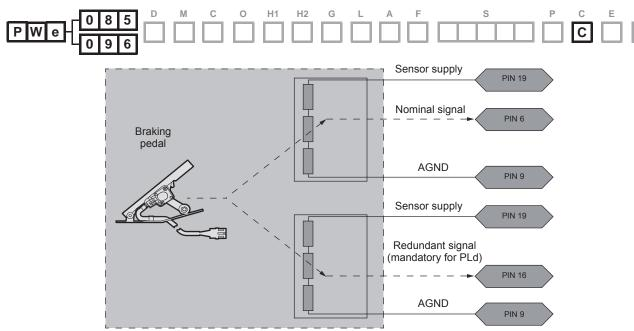
Safety requirements for compliance PLd, the braking pedal must:
