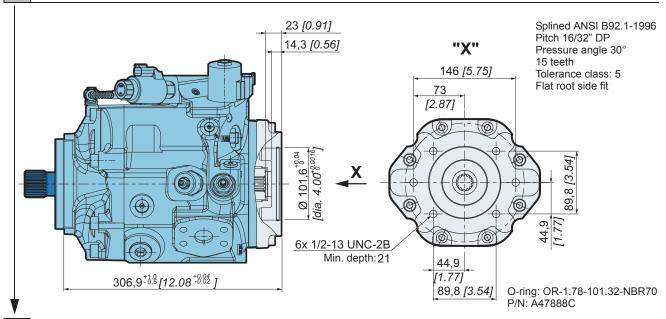
SAE-C; Coupling torque: 701 Nm [6204 in.lbf]; minimum active spline lenght: 14,5 mm [0.57 inch]
