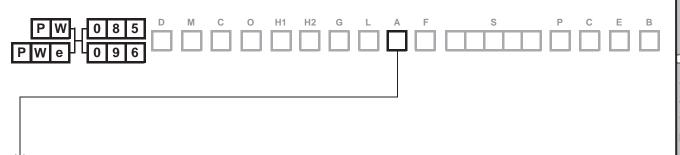
SAE-BB; Coupling torque: 407Nm [3602 in.lbf]; minimum active spline lenght: 13 mm [0.51 inch]
