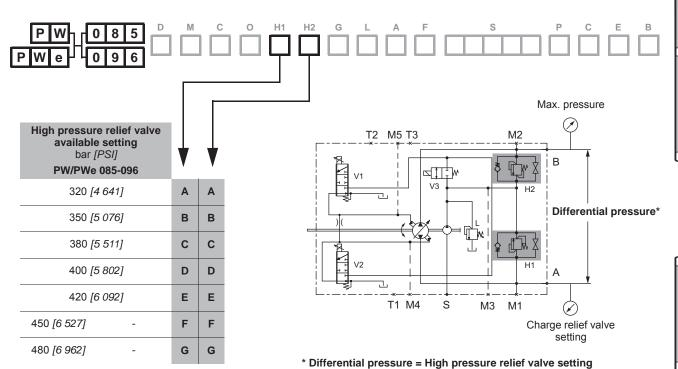
(Max. pressure = HPRV setting + CPRV setting)
