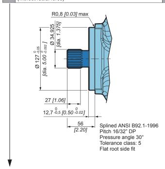
R0,8 [0.03] max 38, ldia. Ø -0.002 J Ø 127-0,05 [dia. 5.00] 27 [1.06] 12,7 -0,5 [0.50 -0.02] 56 Splined ANSI B92.1-1996 [2.20] Pitch 16/32" DP Pressure angle 30° Tolerance class: 5 Flat root side fit
