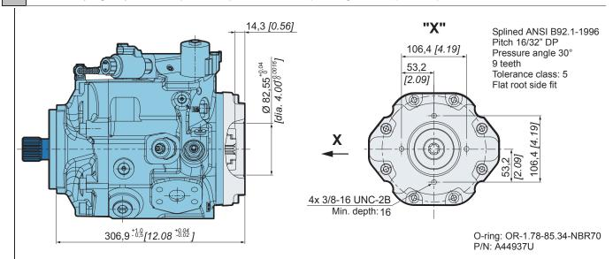
SAE-B; Coupling torque: 283 Nm [2505 in.lbf]; minimum active spline lenght: 12 mm [0.47 inch]
