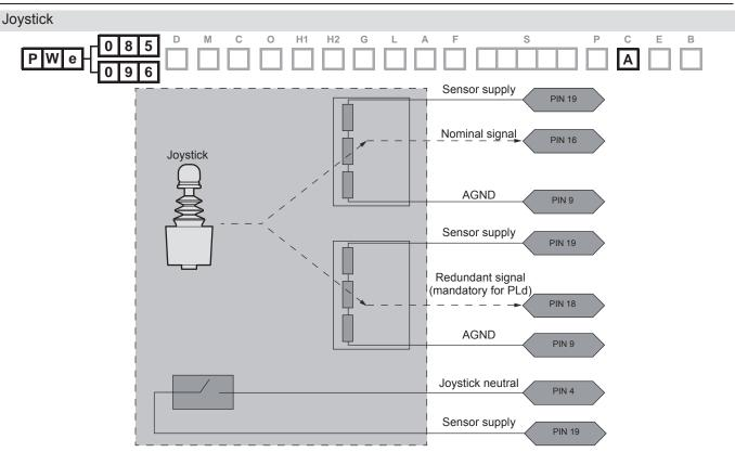
Safety requirements for compliance PLd, the joystick must:
