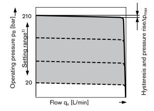
1) In order to prevent damage to the pump and the system the shown values in the pressure setting range are the maximum permissible and may not be exceede.
