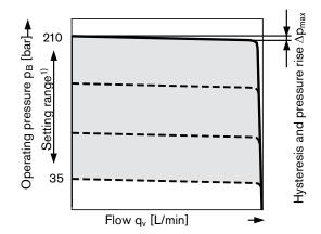
1) In order to prevent damage to the pump and the system the shown values in the pressure setting range are the maximum permissible and may not be exceede.
