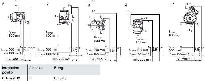
$L/L_1$  = case drain port, F = air bleed or filling port, S = suction port, SB = Baffle,  $h_{t min}$  = minimum permissible immersion depth,  $h_{S max}$  = maximum permissible suction height
