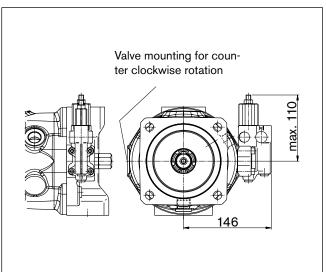
DRG - Pressure control, remotely operated
